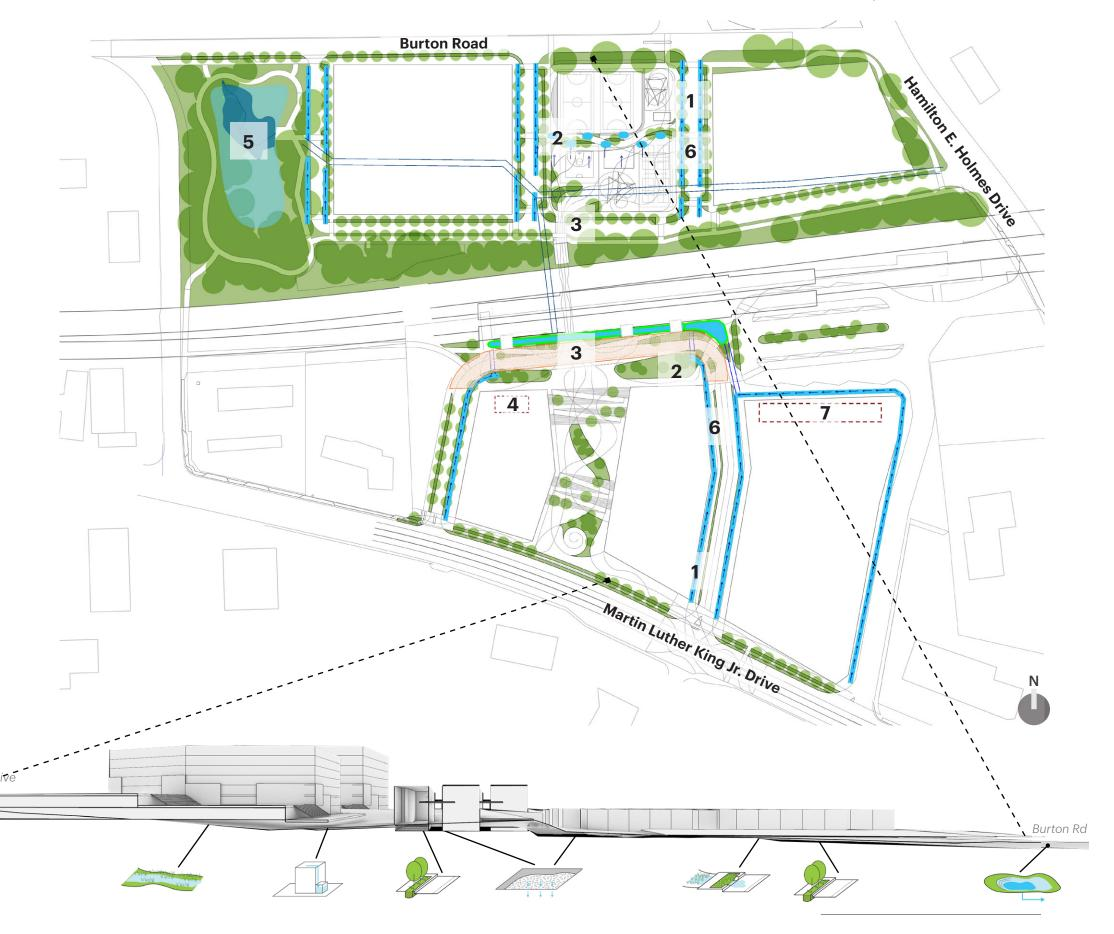
Bioretention strips along station front and entry area
